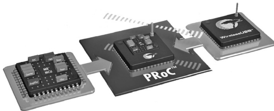
Figure 8.2 A conceptual representation of Cypress WirelessUSB solution with PRoC flash programmable microcontroller and integrated 2.4GHz radio transceiver.
